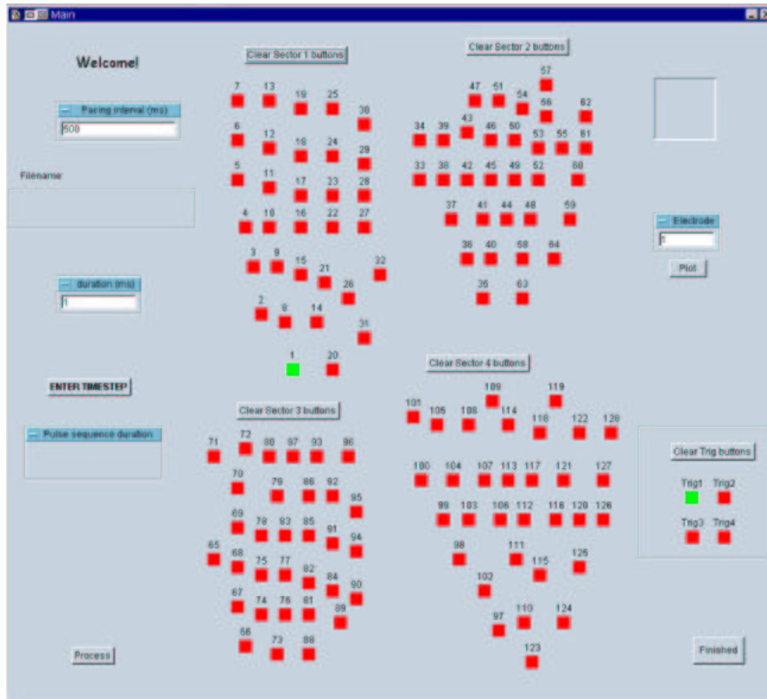
Figure 2.5: Screenshot of the PaceGUI application. Icons representing all 128 electrodes are laid out on screen.
