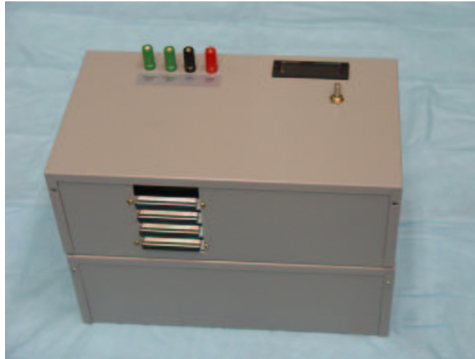
Figure 2.4: Photograph of pacing boxes, which housed the power supply and the custom-made circuit boards. Connections coming from the computer and connections going to the electrode sock were in the back and front of the boxes, respectively.
