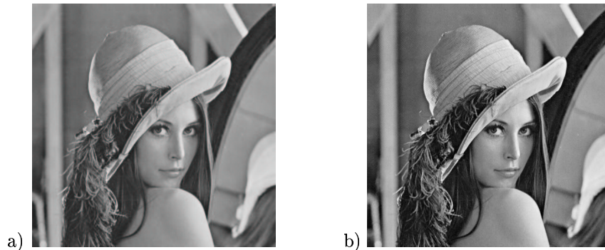
Figure 2: Demonstration of images using Method 2 algorithm. (a) Original Lena image, (b) water-marked Lena. PSNR = 43.4dB
